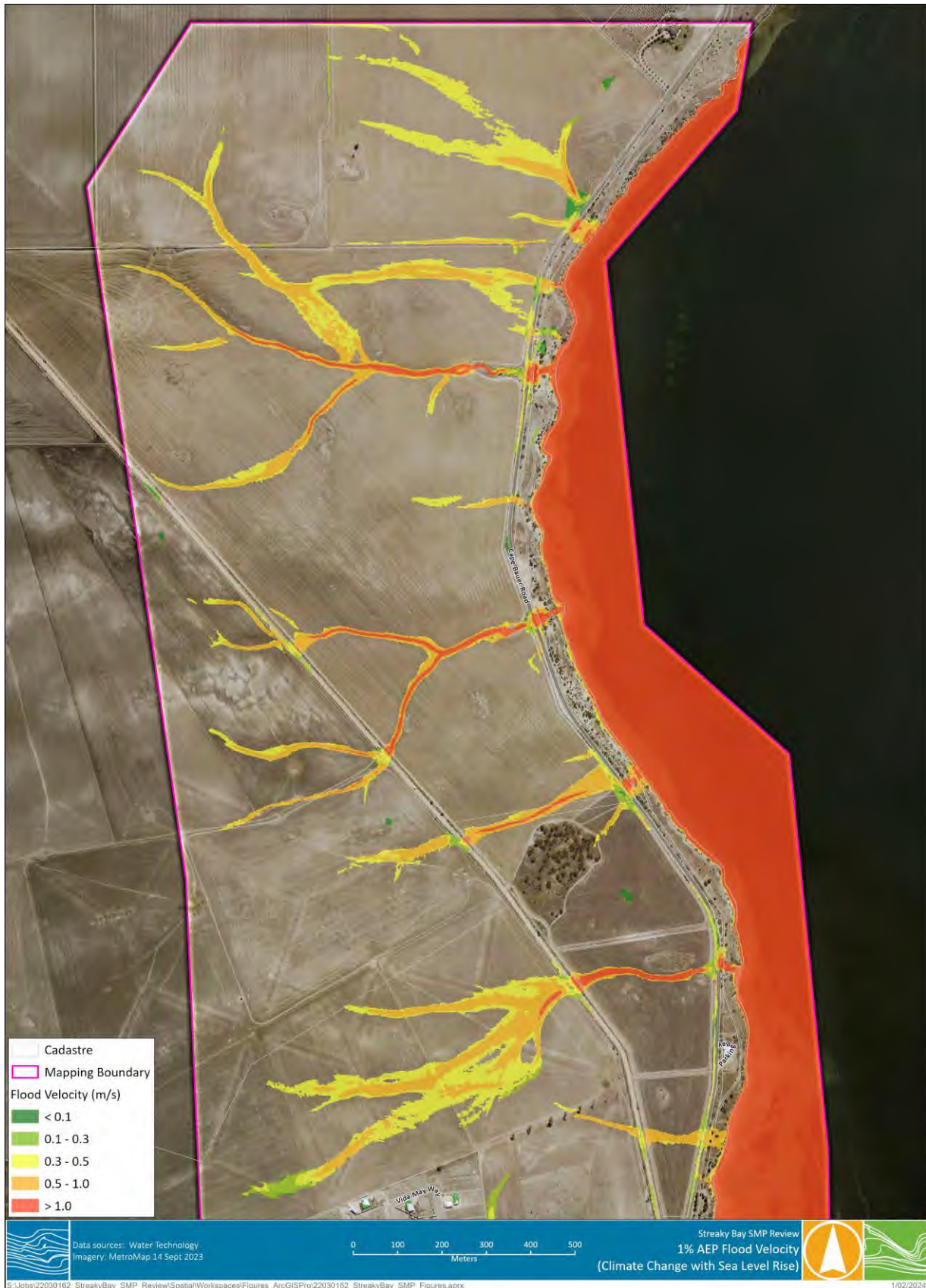
Figure D-3 Future Conditions (Climate Change with Sea Level Rise) – 1% AEP Flood Velocities
