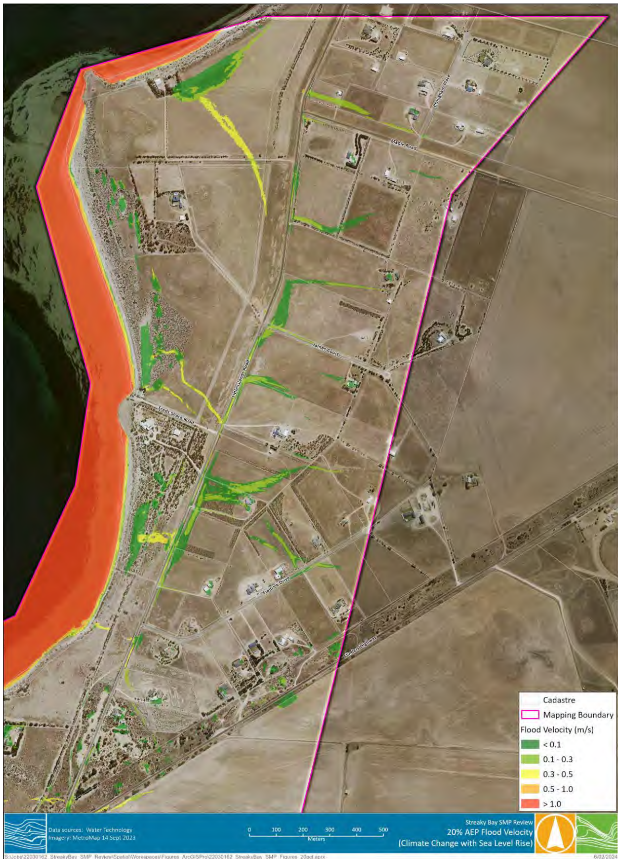
Figure D-14 Future Conditions (Climate Change with Sea Level Rise) – 20% AEP Flood Velocities
