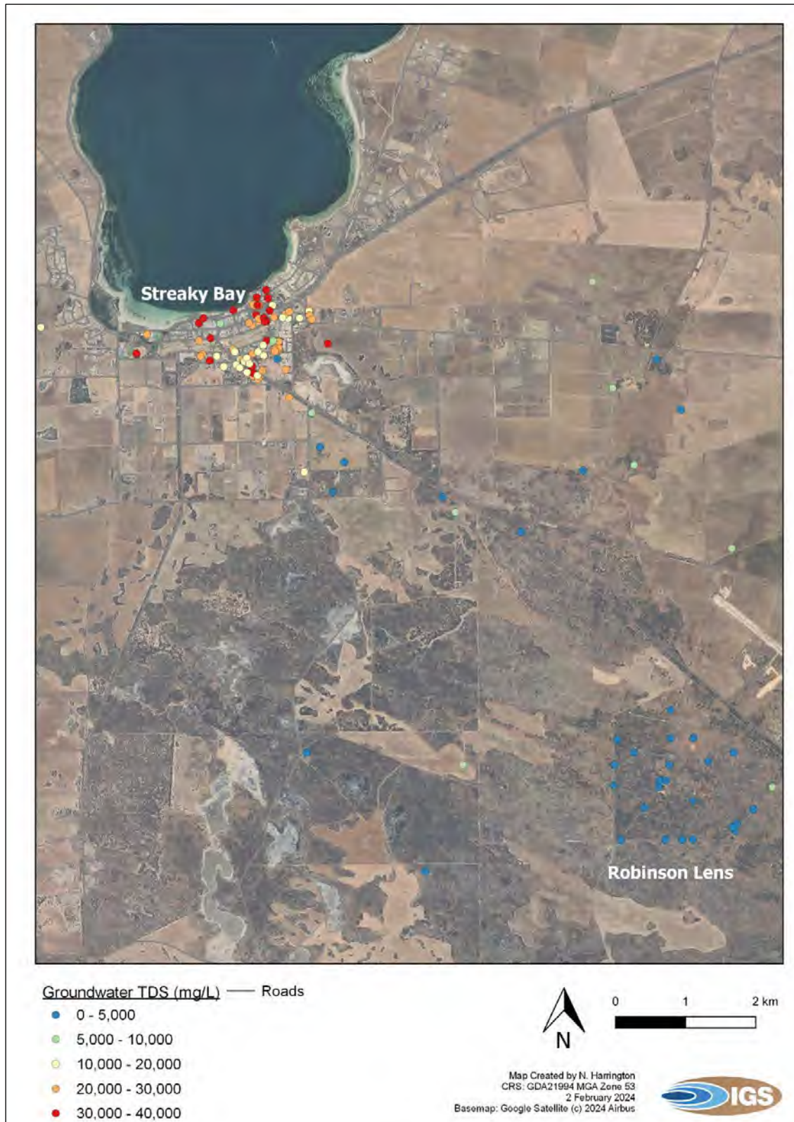
Figure A-18 Latest Groundwater Salinities (TDS) as Listed on the WaterConnect Database (main dataset) and from a recent Groundwater Monitoring Program carried out at Robinson Lens (IGS, 2023)
