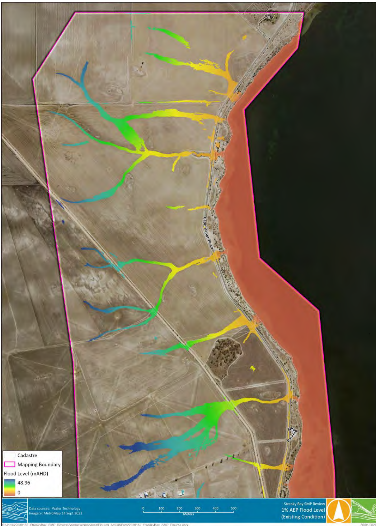
Figure B-1 Existing Conditions - 1% AEP Flood Levels
