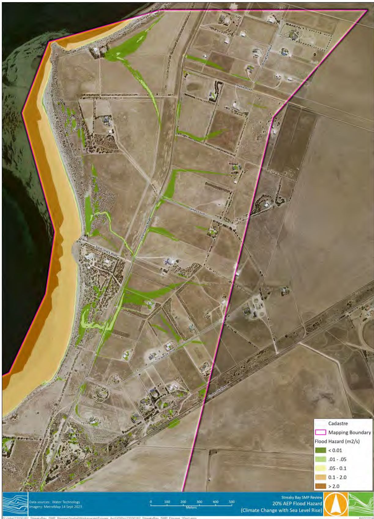
Figure D-15 Future Conditions (Climate Change with Sea Level Rise) – 20% AEP Flood Hazards
