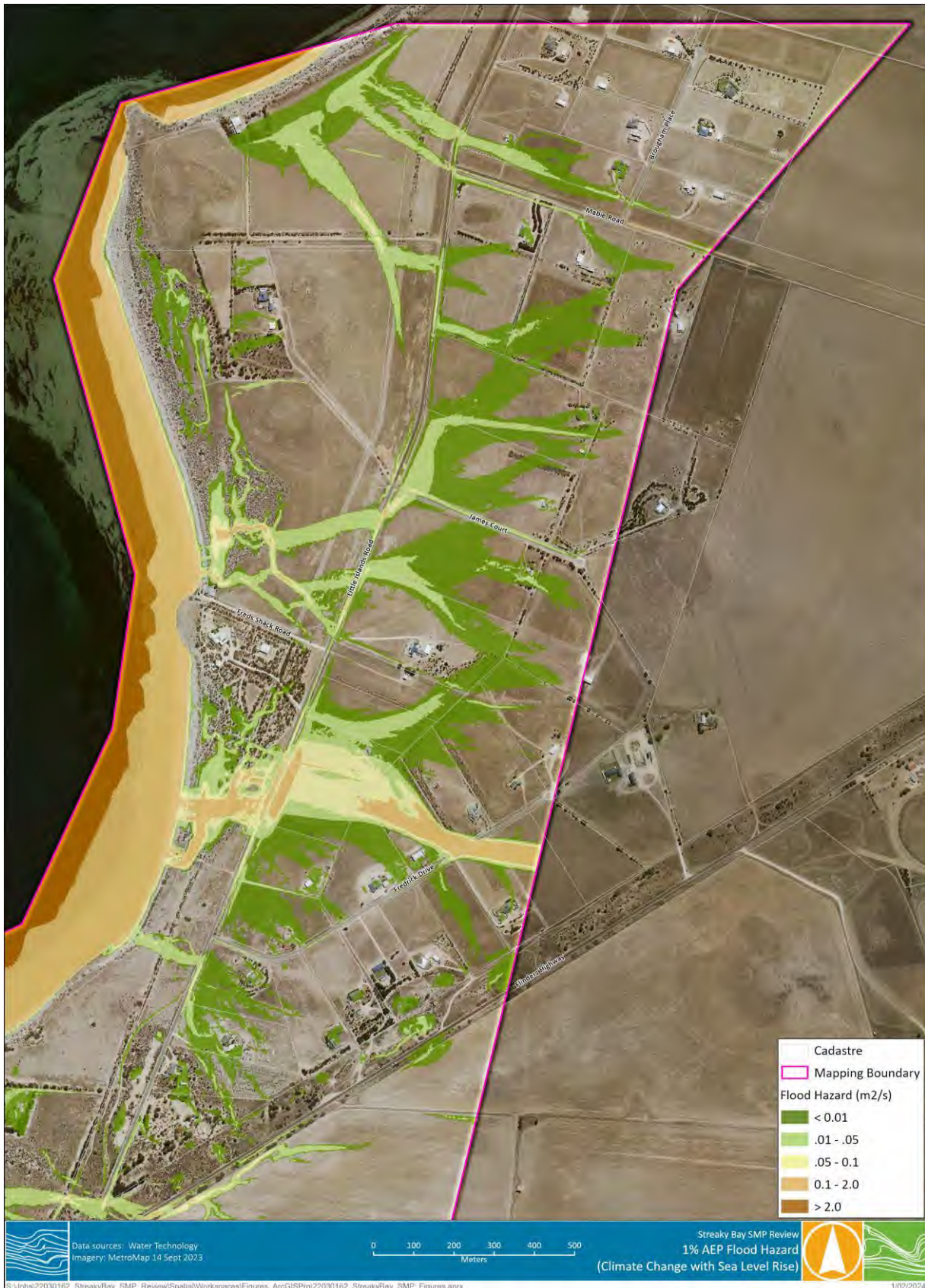
Figure D-12 Future Conditions (Climate Change with Sea Level Rise) – 1% AEP Flood Hazards
