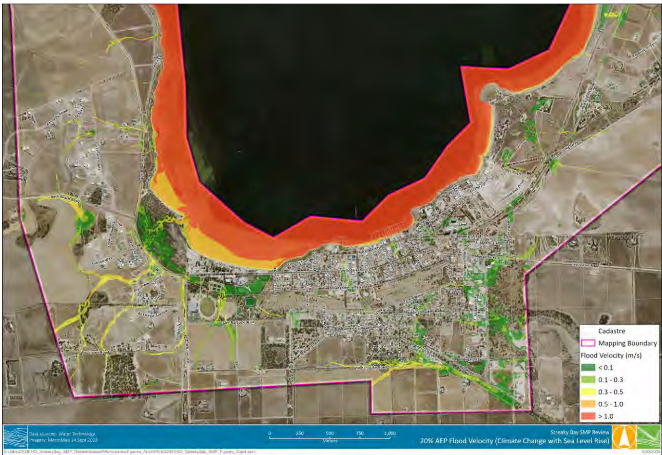
Figure D-22 Future Conditions (Climate Change with Sea Level Rise) – 20% AEP Flood Velocities
