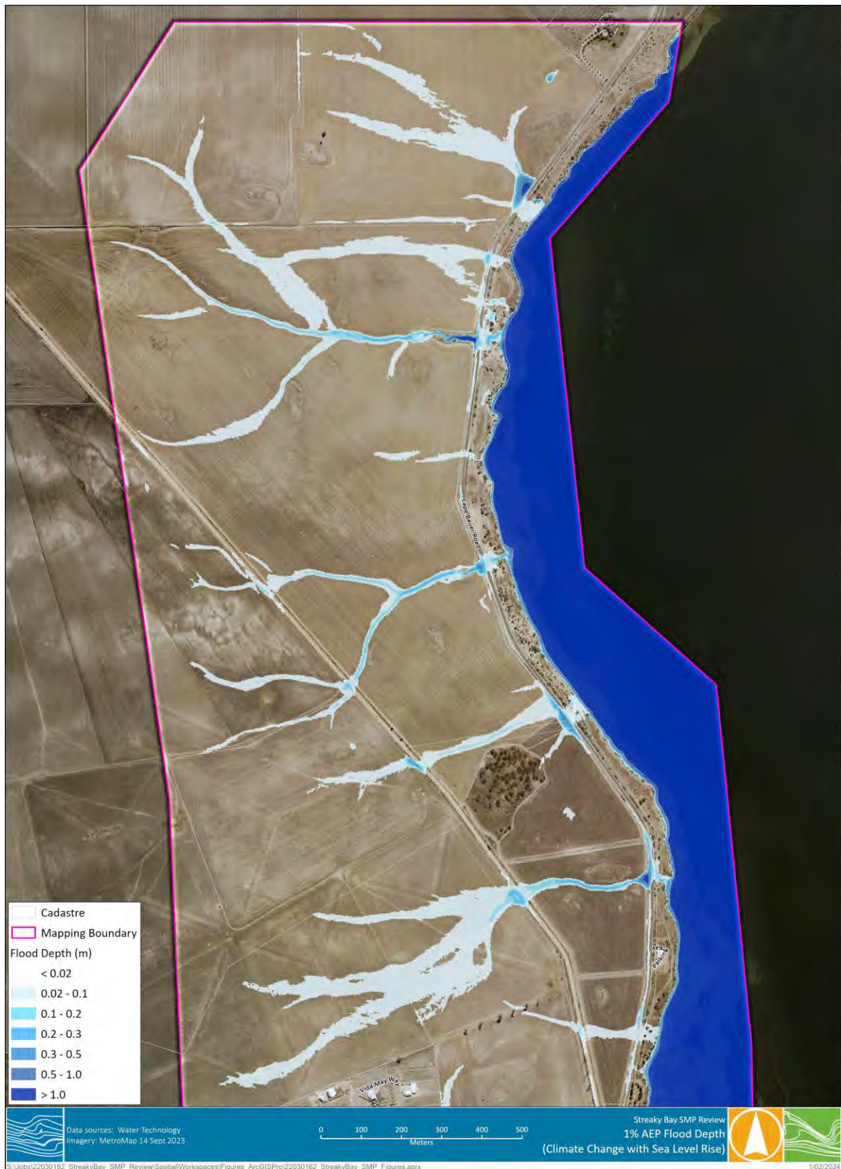
Figure D-2 Future Conditions (Climate Change with Sea Level Rise) – 1% AEP Flood Depths
