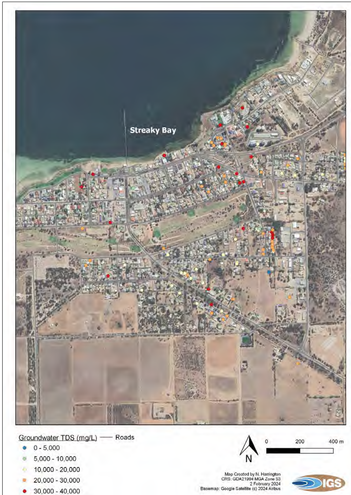
Figure A-19 Latest Groundwater Salinities (TDS) as Listed on the WaterConnect Database for the Streaky Bay Township Area
