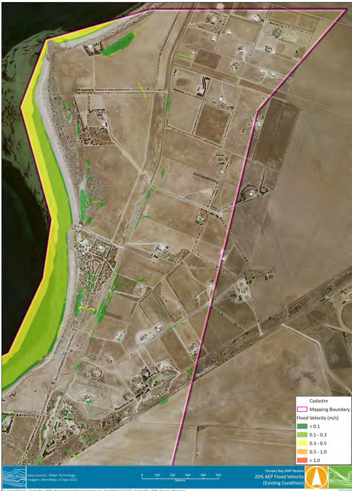
Figure B-23 Existing Conditions - 20% AEP Flood Velocities
