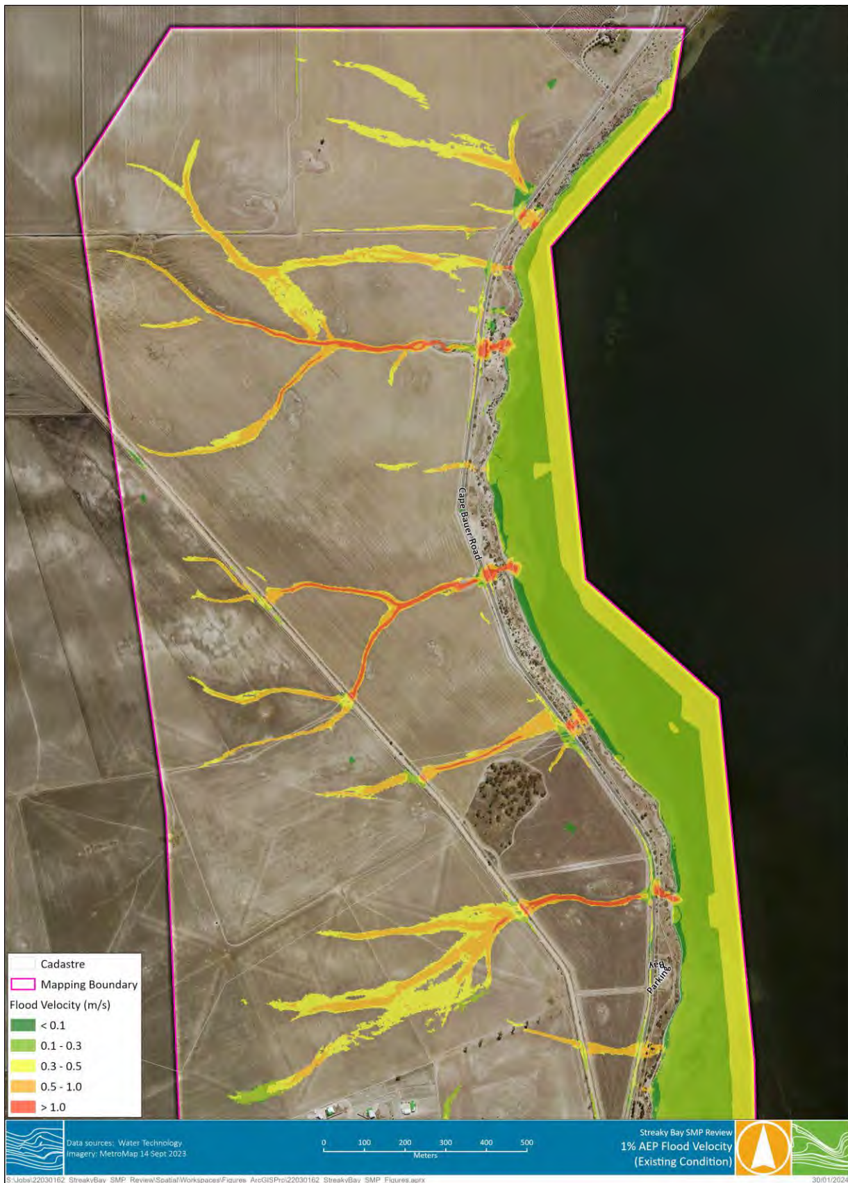
Figure B-3 Existing Conditions - 1% AEP Flood Velocity
