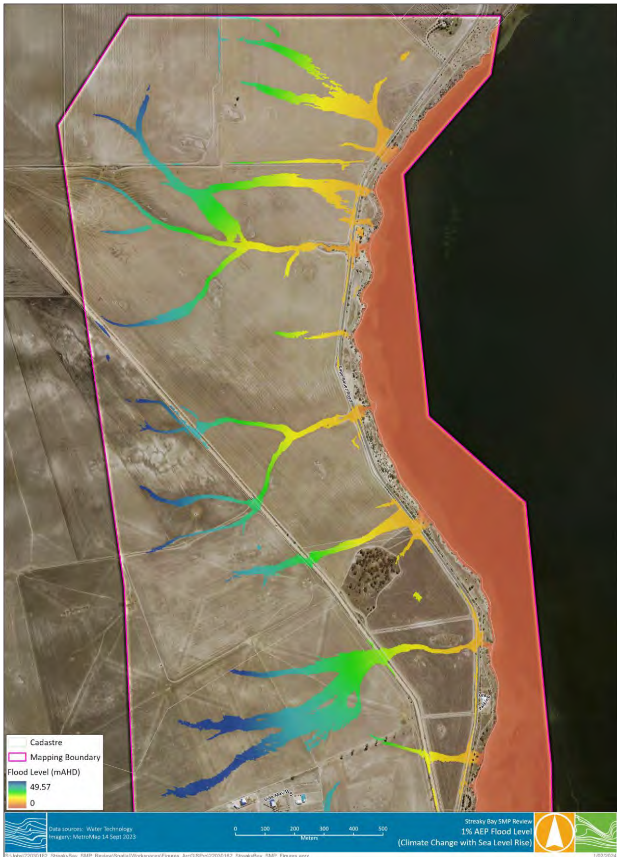
Figure D-5 Future Conditions (Climate Change with Sea Level Rise) – 1% AEP Flood Levels
