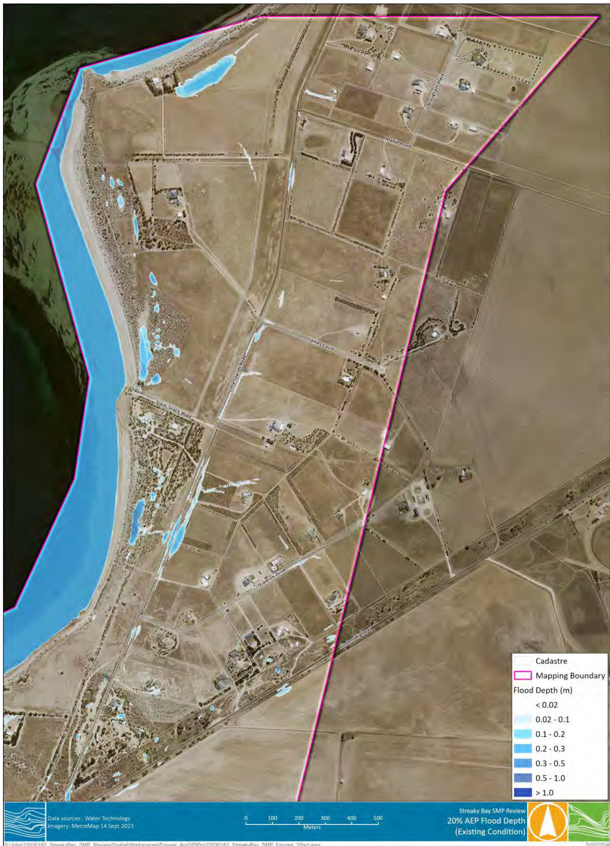
Figure B-22 Existing Conditions - 20% AEP Flood Depths
