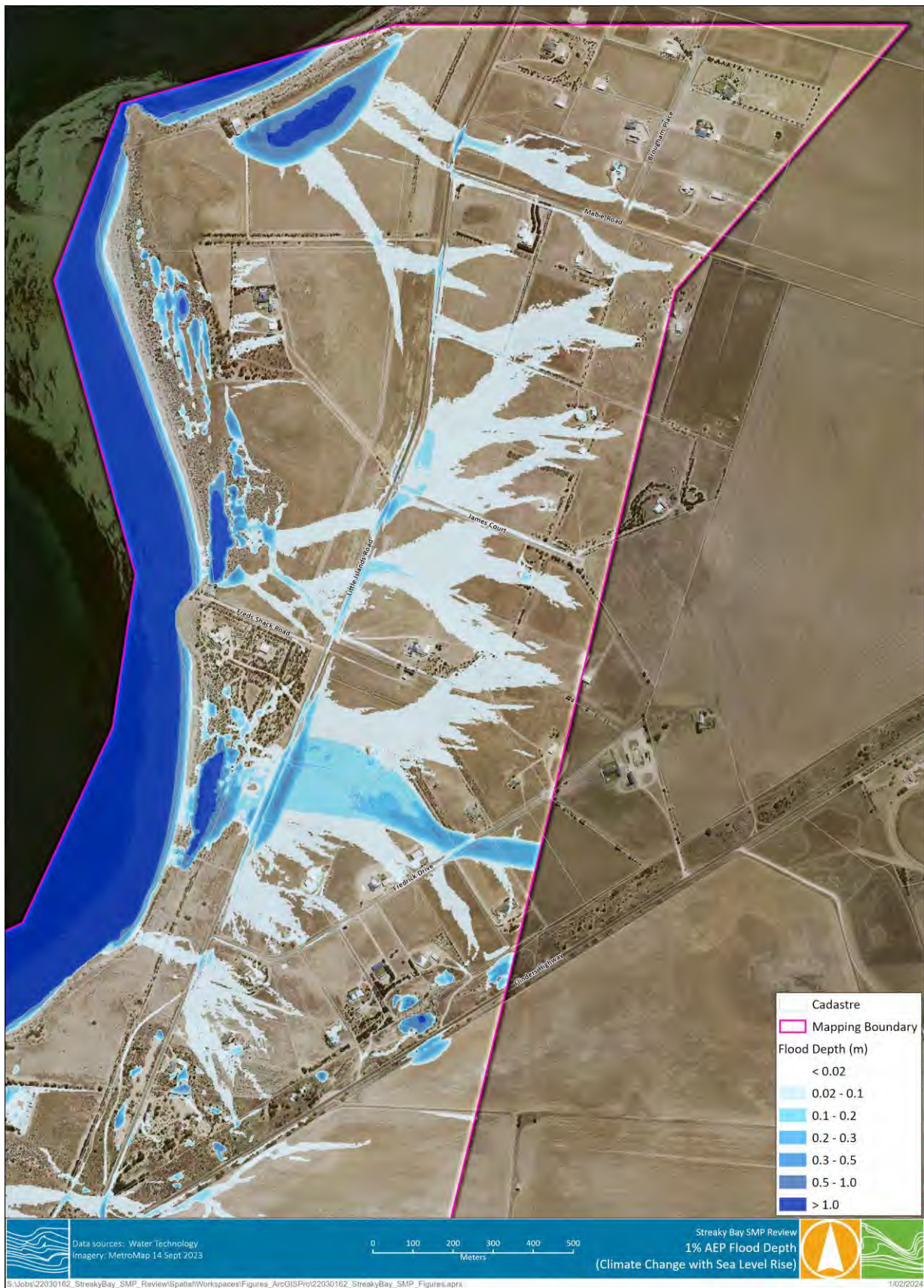
Figure D-10 Future Conditions (Climate Change with Sea Level Rise) – 1% AEP Flood Depths
