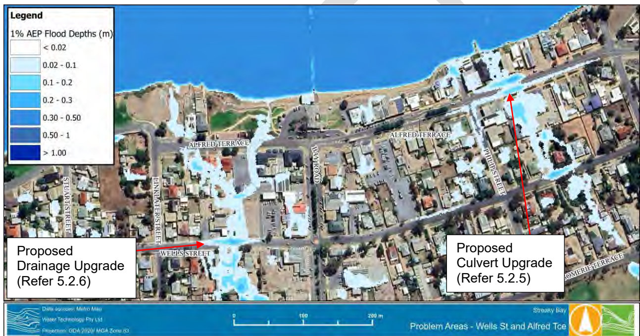
Figure 5-3 Areas along Wells Street and Alfred Terrace subject to inundation
