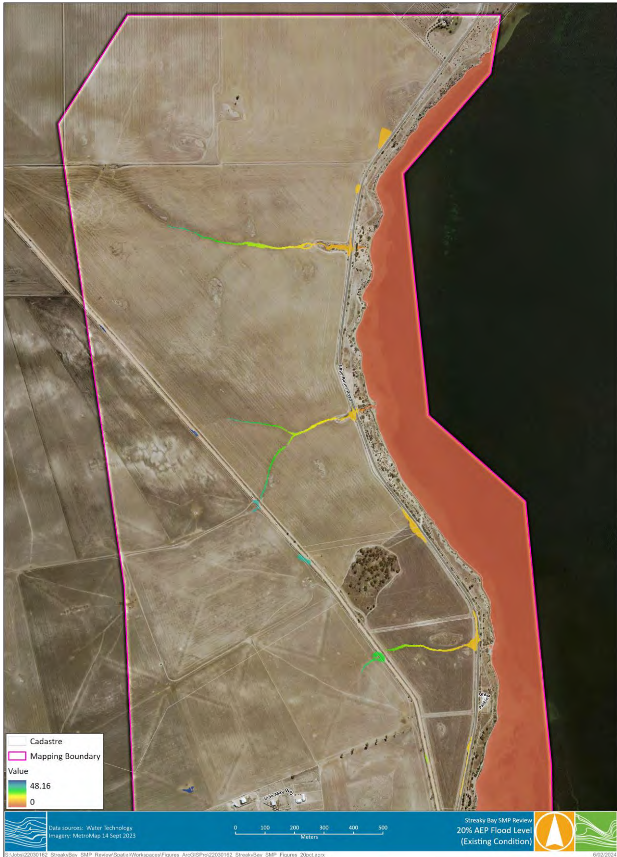
Figure B-17 Existing Conditions - 20% AEP Flood Levels
