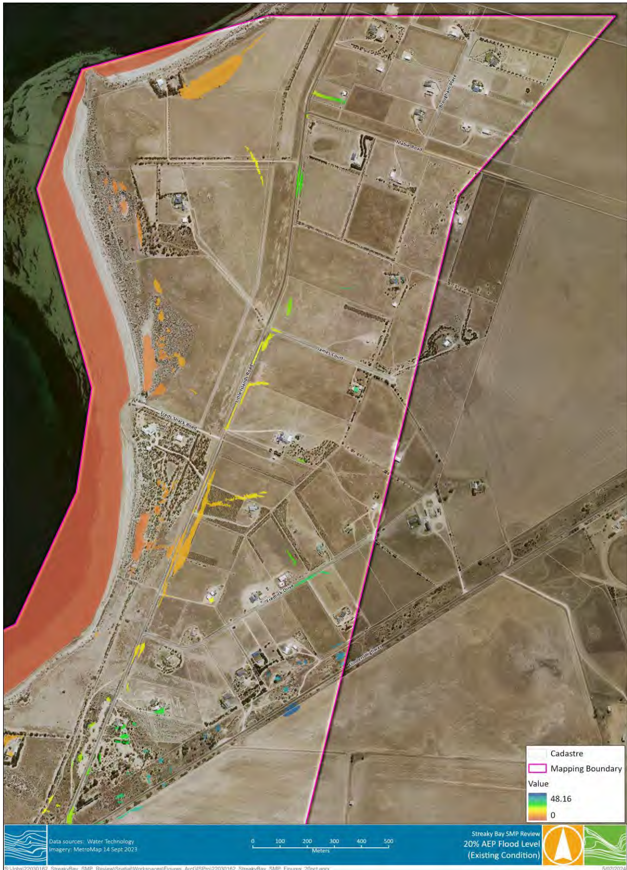
Figure B-13 Existing Conditions - 20% AEP Flood Levels
