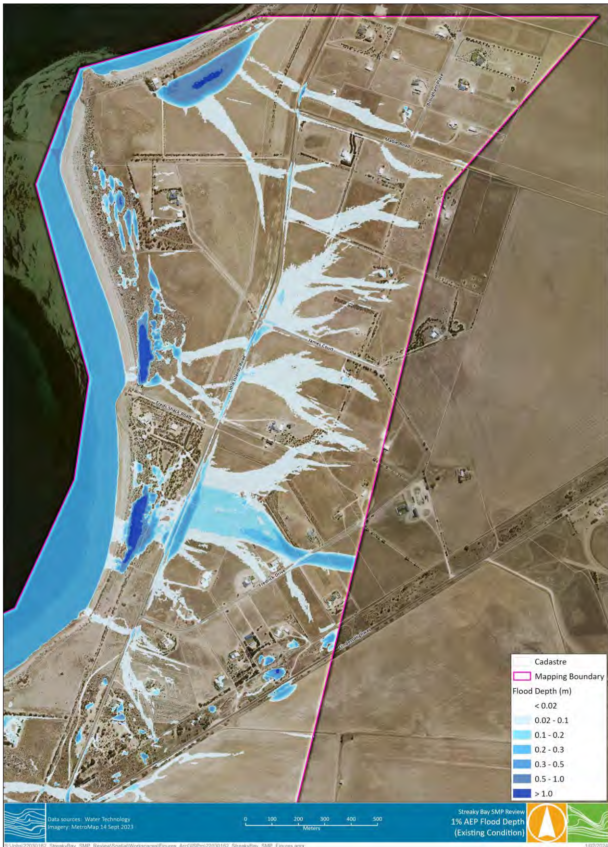
Figure B-8 Existing Conditions - 1% AEP Flood Depths
