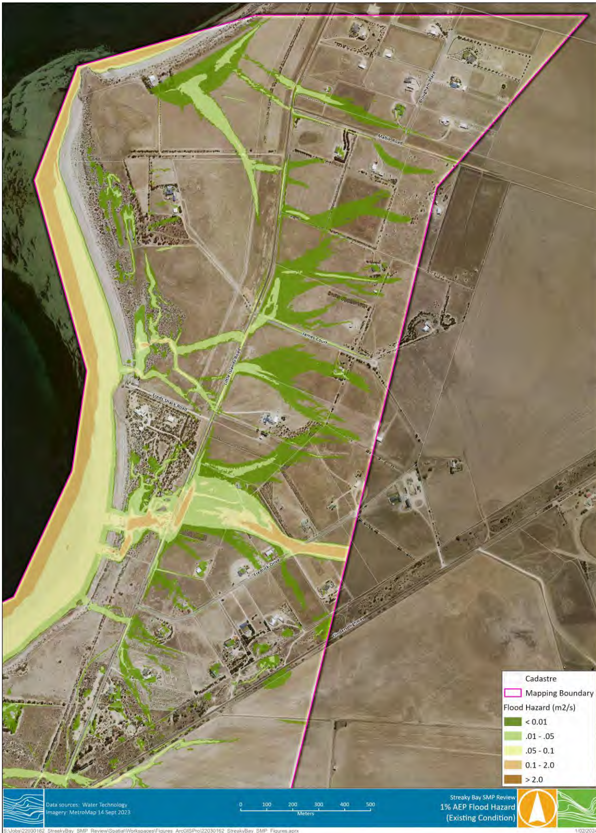
Figure B-10 Existing Conditions - 1% AEP Flood Hazards
