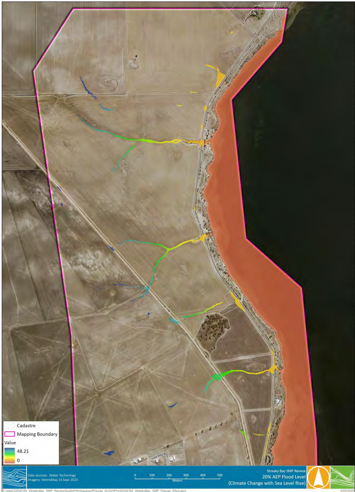
Figure D-20 Future Conditions (Climate Change with Sea Level Rise) – 20% AEP Flood Levels
