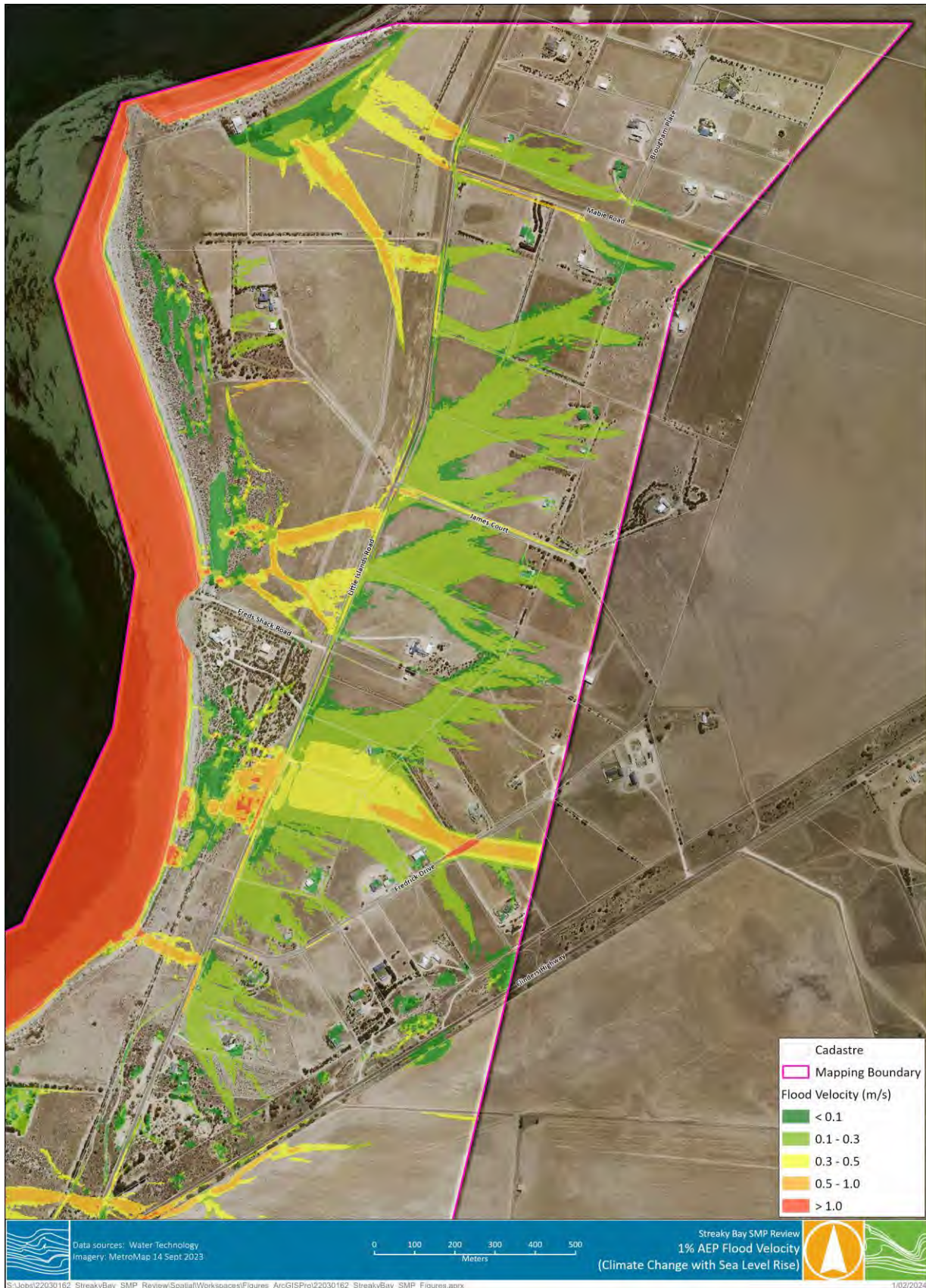
Figure D-11 Future Conditions (Climate Change with Sea Level Rise) – 1% AEP Flood Velocities
