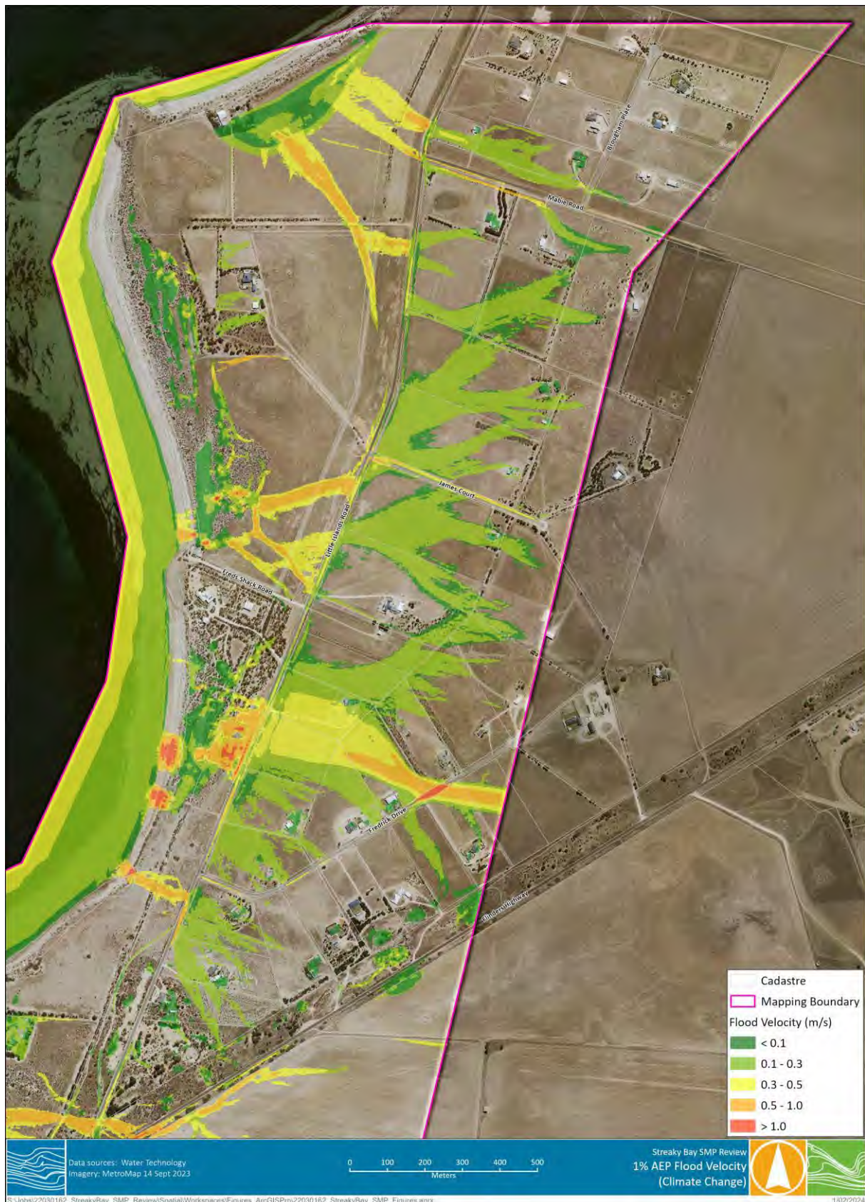
Figure C-12 Future Conditions (Climate Change) – 1% AEP Flood Velocities
