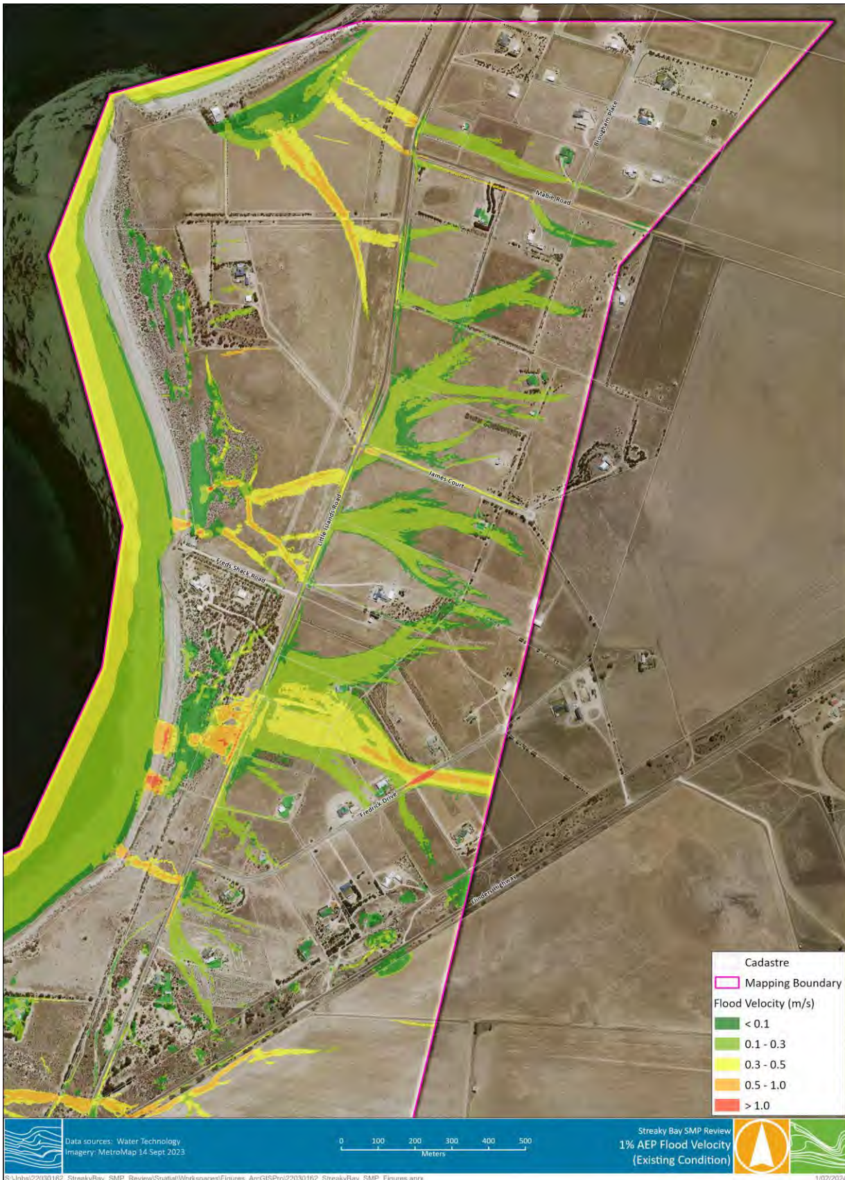
Figure B-9 Existing Conditions - 1% AEP Flood Velocities
