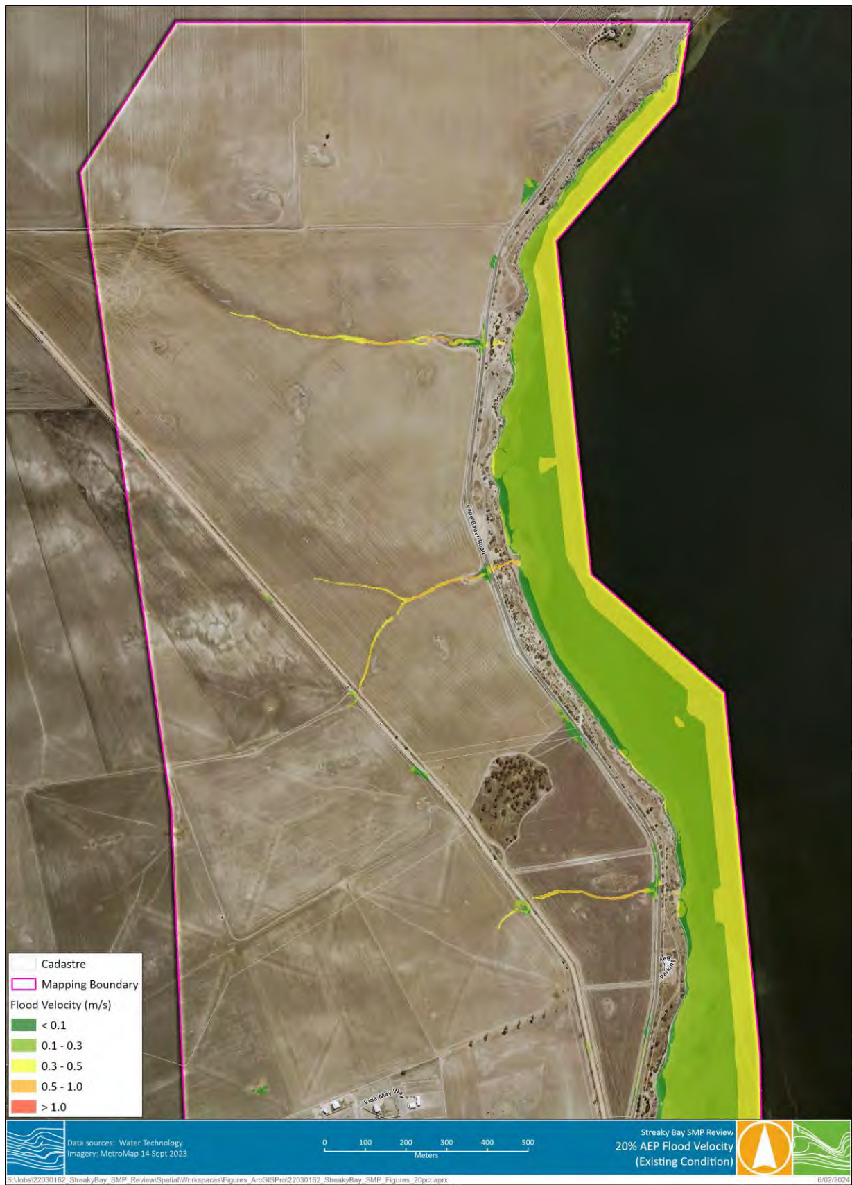
Figure B-15 Existing Conditions - 20% AEP Flood Velocities
