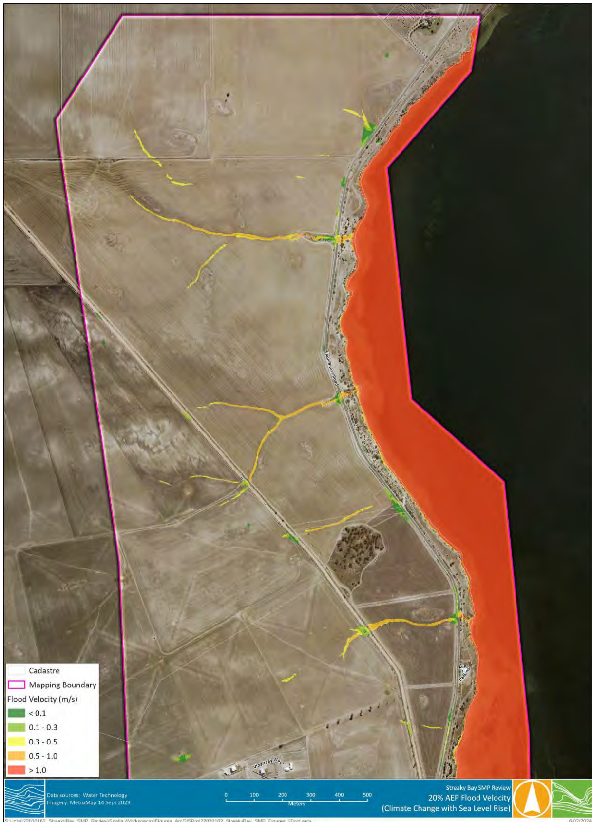
Figure D-18 Future Conditions (Climate Change with Sea Level Rise) – 20% AEP Flood Velocities
