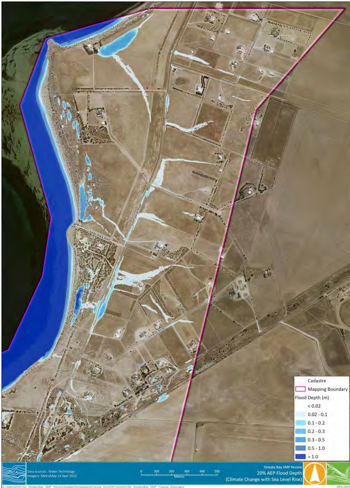
Figure D-13 Future Conditions (Climate Change with Sea Level Rise) – 20% AEP Flood Depths
