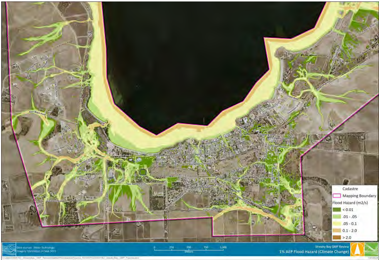
Figure C-9 Future Conditions (Climate Change) – 1% AEP Flood Hazards
