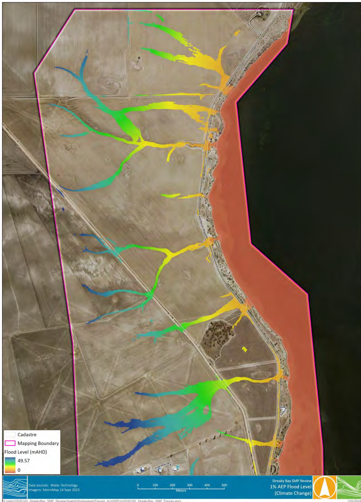
Figure C-6 Future Conditions (Climate Change) – 1% AEP Flood Levels
